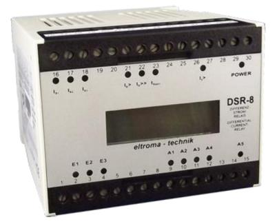
The DSR-8 is a device for measurement and monitoring of differential current at generators, motors and transformers. As well possible is the monitoring of mixed constructions, such as a generator with an upstream transformer. In addition to the differential current, it is also possible to measure the individual conductor currents as well as the earth current in three-wire networks. The connection to the system must be done using external current transformers.
