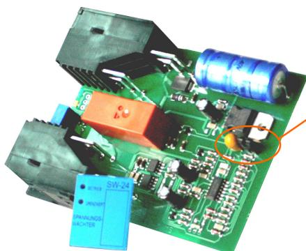
The pre-adjusted delay time can be changed by a jumper on the board of the dismantled SW-12 / 24 unit from 60 seconds (jumper on) to 180 seconds (jumper off).
