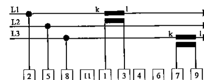
Three-conductor three-phase, asymmetric load 2p3
